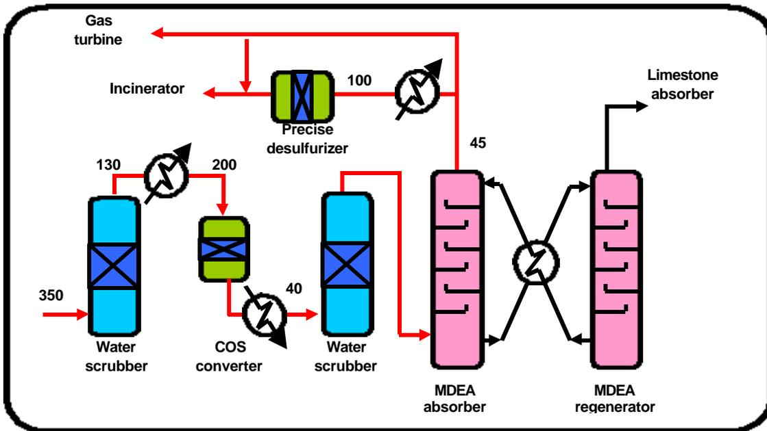
Figure 3 Flow Diagram of Gas Clean-up Unit
