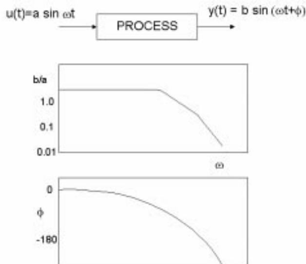
Frequency-dependent (Filtering) Characteristic of a Process
