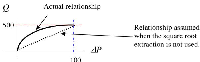
As we can see below, by converting  $\Delta P$  signal linearly into flow rate without the square root extraction, the final reading will be accurate only at the zero flow rate and the maximum flow rate. In the middle, the reading will underestimate the actual flow rate. See that this is true by setting the flow rate at various values and comparing them with the final readings.
