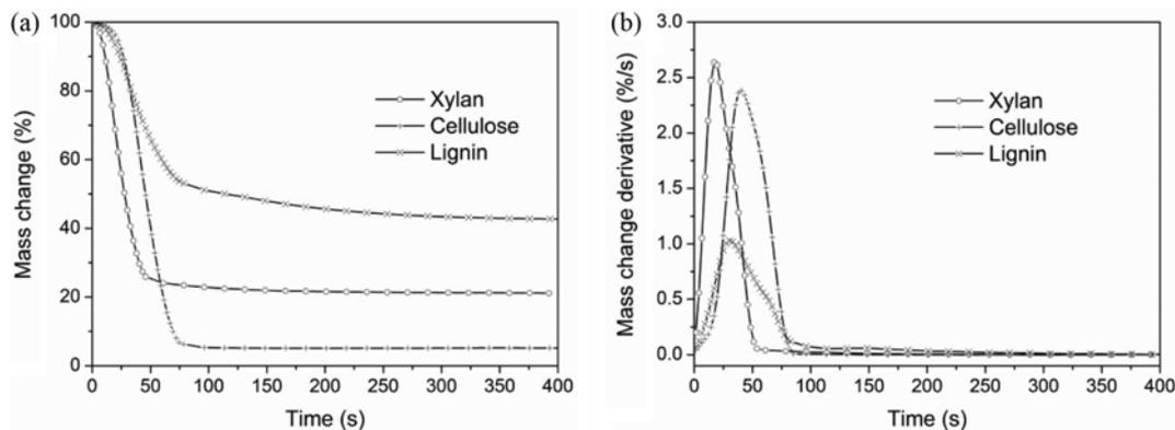
Fig. 3. TG and DTG curves of pyrolysis of xylan, cellulose, and lignin in Macro-TGA.
