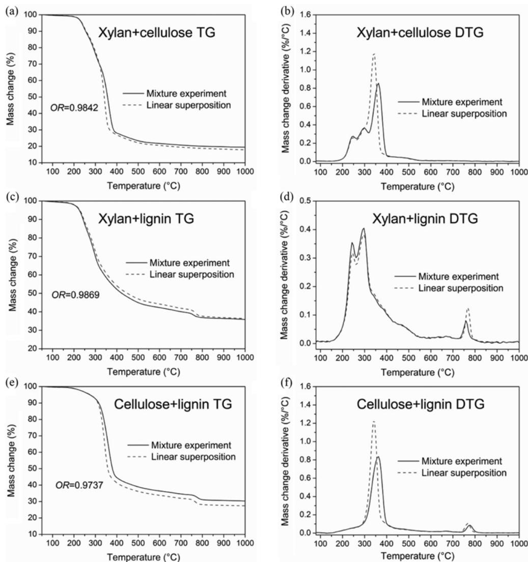
Fig. 4. The comparison of mixture experiments and linear superposition of pyrolysis in TGA.
