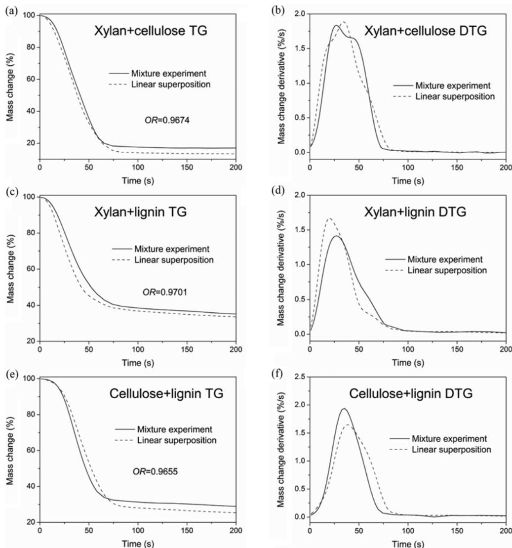
Fig. 5. The comparison of mixture experiments and linear superposition of pyrolysis in Macro-TGA.
