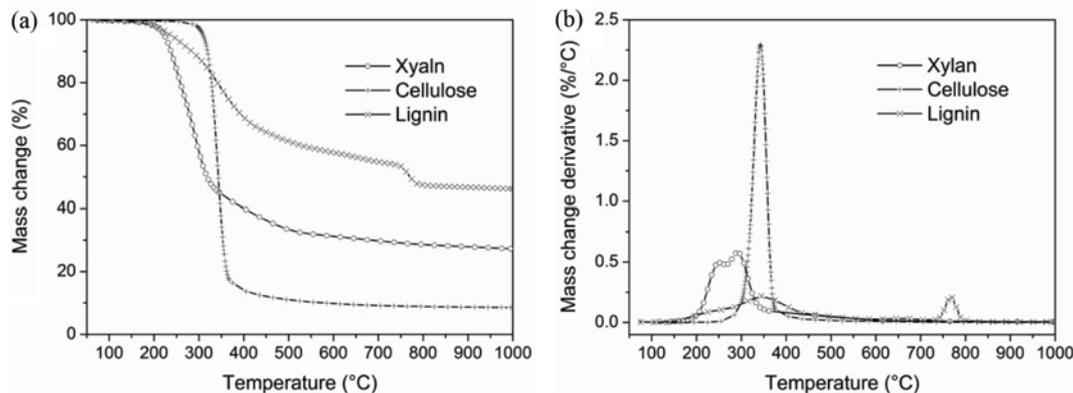
Fig. 2. TG and DTG curves of pyrolysis of xylan, cellulose, and lignin in TGA.
