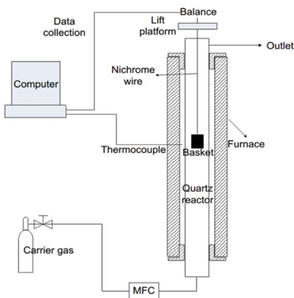
**Fig. 1. Schematic diagram of Macro-TGA system.**
