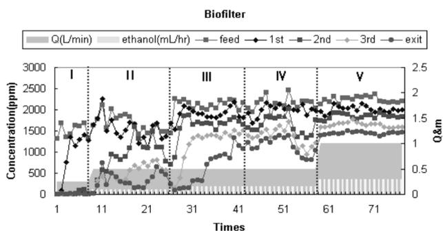
**Fig. 4. Various ethanol concentrations of biofilter at each sampling port versus experimental times.**
