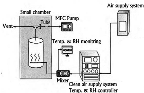
Figure 2. Schematic diagram of small chamber test system.
