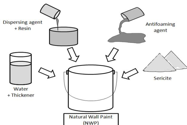
Figure 1. Schematic representation for the preparation of natural wall paint (NWP).
