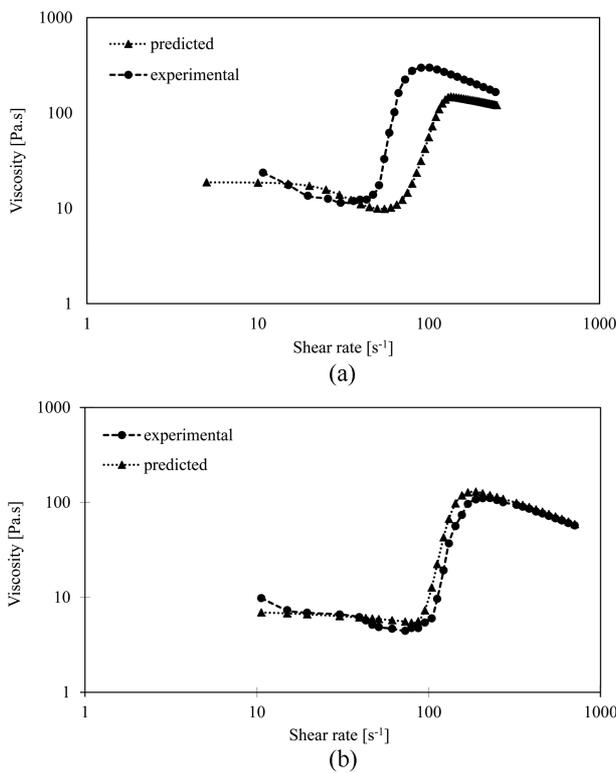
**Fig. 5.** Experimental and predicted viscosity by phenomenological model for testing data sets corresponding to (a) 15°C, and (b) 25°C.
