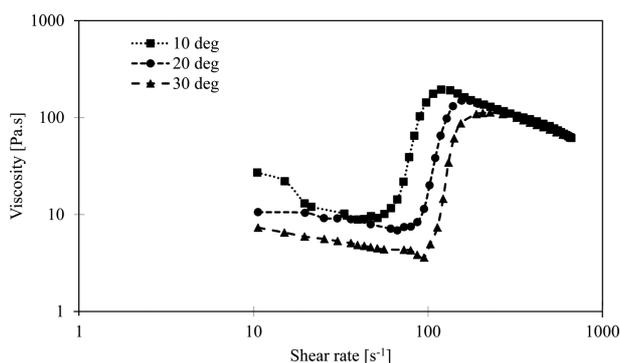
**Fig. 3.** Rheological behavior of 65% STF at different temperatures.
