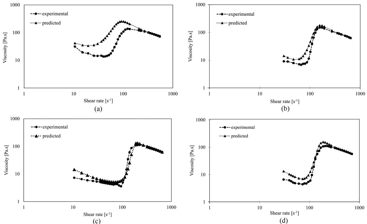
**Fig. 6.** Experimental and predicted viscosity by ANN model for training data sets (a) 10°C, (b) 20°C, (c) 30°C, and (d) testing data set 25°C.
