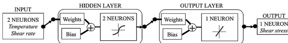
Fig. 2. ANN architecture designed for the prediction of shear stress of STF.
