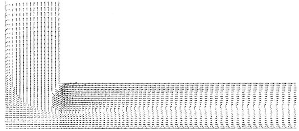
Fig. 7. Typical fiber orientation around sprue junction region.
