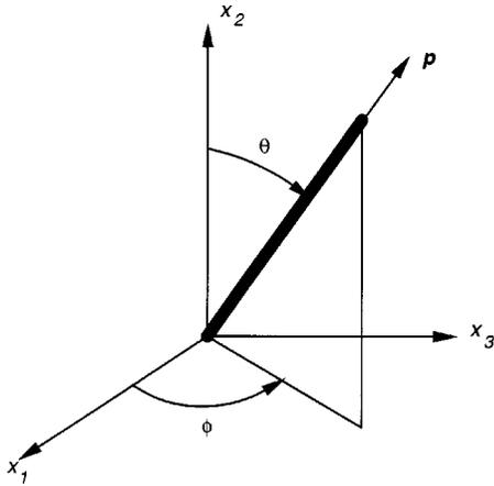
Fig. 1. Orientation of a single fiber.
