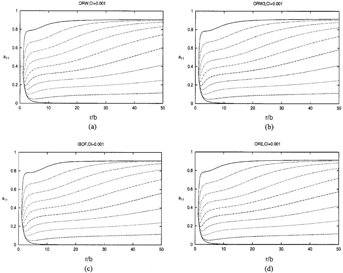
**Fig. 4.**  $a_{11}$  component in isothermal Newtonian radial diverging flow as a function of radial location ( $r/b$ ) at several thickness positions ( $z/b$ ) for various closure approximations with  $C_I=0.001$ : (a) ORW, (b) ORW3, (c) IBOF, (d) ORE. The meaning of curves is the same as that in Fig. 3.
