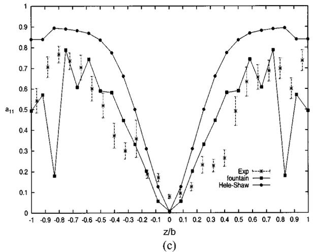
**Fig. 10.** Effect of fountain flow vs. Hele-Shaw (lubrication approximation) on  $a_{11}$  component for non-Newtonian fiber suspension flow (fiber-fluid decoupled case,  $C_f=0.001$ ) as a function of thickness positions ( $z/b$ ) for center-gated disk; (a) at  $r/b=5.68$  (b) at  $r/b=22.8$  (c) at  $r/b=40.4$ .
