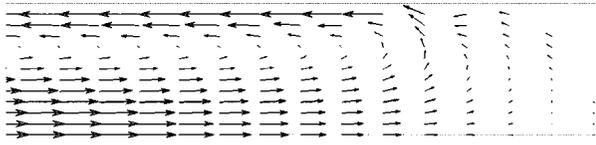
**Fig. 9.** Predicted velocity plot showing fountain flow around melt front region for non-Newtonian fiber suspension flow (fiber-fluid decoupled case,  $C_f=0.001$ ). Reference frame is moving with the melt front and the length of arrow indicates relative magnitude of the velocity.
