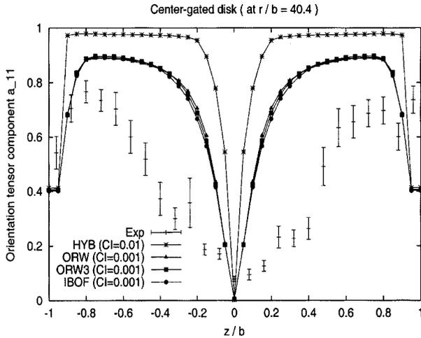
**Fig. 6.**  $a_{11}$  (flow-directional orientation) component as a function of thickness positions ( $z/b$ ) for various closure approximations of HYB, ORW, ORW3 and IBOF with experimental data for center-gated disk at  $r/b=40.4$ .
