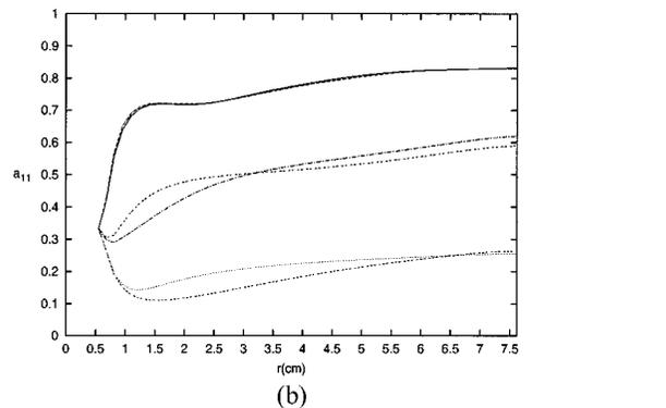
Fig. 8. Coupling effect on  $a_{11}$  component for isothermal Newtonian flow ( $C_f=0.001$ ) as a function of radial positions ( $r$ ) for center-gated disk (a) including fountain flow (b) neglecting fountain flow.
