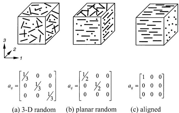
Fig. 2. Example of different orientation states and corresponding orientation tensors.
