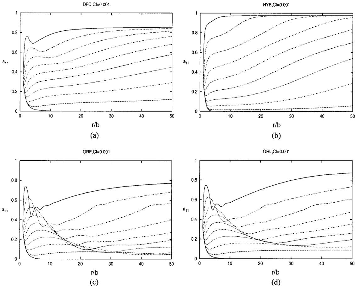
**Fig. 3.**  $a_{11}$  component in isothermal Newtonian radial diverging flow as a function of radial location ( $r/b$ ) at several thickness positions ( $z/b$ ) ( $z/b = 0.9, 0.8, 0.7, 0.6, 0.5, 0.4, 0.3, 0.2, 0.1, 0.0$  from the top to bottom curves) for various closure approximations with  $C_I=0.001$ : (a) DFC, (b) HYB, (c) ORF, (d) ORL.
