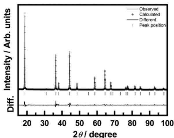
**Figure 2.** X-ray Rietveld refined pattern of Li[Ni<sub>0.5</sub>Co<sub>0.05</sub>Mn<sub>1.45</sub>]O<sub>4</sub> material.
