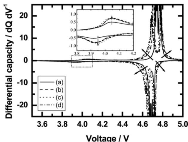
**Figure 5.** Differential capacity vs. voltage curves for Li/Li[Ni<sub>0.5</sub>Co<sub>y</sub>Mn<sub>1.5-y</sub>]O<sub>4-z</sub>F<sub>z</sub> cells: (a) Li[Ni<sub>0.5</sub>Mn<sub>1.5</sub>]O<sub>4</sub>, (b) Li[Ni<sub>0.5</sub>Co<sub>0.05</sub>Mn<sub>1.45</sub>]O<sub>4</sub>, (c) Li[Ni<sub>0.5</sub>Co<sub>0.05</sub>Mn<sub>1.45</sub>]O<sub>3.95</sub>F<sub>0.05</sub>, and (d) Li[Ni<sub>0.5</sub>Co<sub>0.1</sub>Mn<sub>1.4</sub>]O<sub>3.9</sub>F<sub>0.1</sub>.
