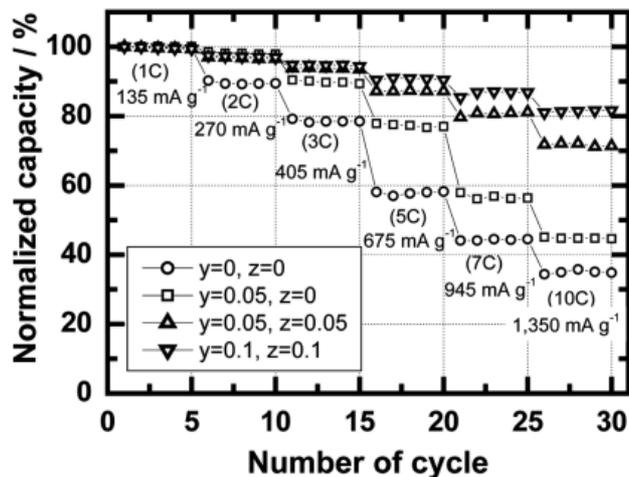
**Figure 7.** Normalized capacity vs. number of cycles for Li/Li $[\text{Ni}_{0.5}\text{Co}_y\text{Mn}_{1.5-y}]\text{O}_{4-z}\text{F}_z$  cells with various current densities between 3.5 and 5.0 V. The cells were charged using a current density of  $27 \text{ mA g}^{-1}$  (0.2 C-rate).
