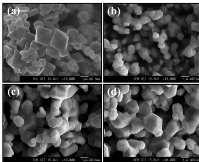
**Figure 3.** SEM images of  $\text{Li}[\text{Ni}_{0.5}\text{Co}_y\text{Mn}_{1.5-y}]\text{O}_{4-z}\text{F}_z$  powders: (a)  $\text{Li}[\text{Ni}_{0.5}\text{Mn}_{1.5}]\text{O}_4$ , (b)  $\text{Li}[\text{Ni}_{0.5}\text{Co}_{0.05}\text{Mn}_{1.45}]\text{O}_4$ , (c)  $\text{Li}[\text{Ni}_{0.5}\text{Co}_{0.05}\text{Mn}_{1.45}]\text{O}_{3.95}\text{F}_{0.05}$ , and (d)  $\text{Li}[\text{Ni}_{0.5}\text{Co}_{0.1}\text{Mn}_{1.4}]\text{O}_{3.9}\text{F}_{0.1}$ .
