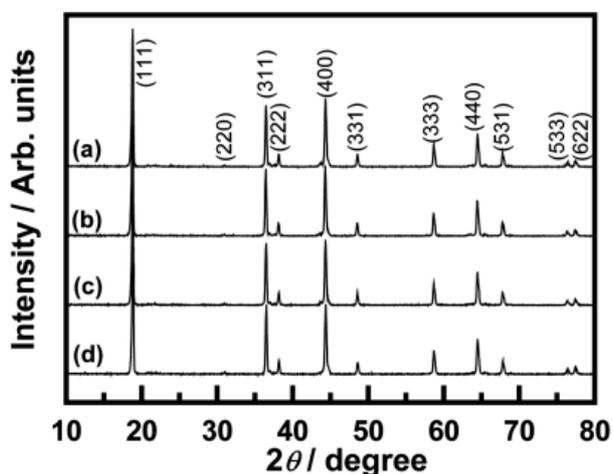
**Figure 1.** X-ray diffraction patterns of Li[Ni<sub>0.5</sub>Co<sub>y</sub>Mn<sub>1.5-y</sub>]O<sub>4-z</sub>F<sub>z</sub> powders: (a) Li[Ni<sub>0.5</sub>Mn<sub>1.5</sub>]O<sub>4</sub>, (b) Li[Ni<sub>0.5</sub>Co<sub>0.05</sub>Mn<sub>1.45</sub>]O<sub>4</sub>, (c) Li[Ni<sub>0.5</sub>Co<sub>0.05</sub>Mn<sub>1.45</sub>]O<sub>3.95</sub>F<sub>0.05</sub>, and (d) Li[Ni<sub>0.5</sub>Co<sub>0.1</sub>Mn<sub>1.4</sub>]O<sub>3.9</sub>F<sub>0.1</sub>.
