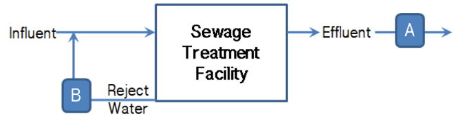
Fig. 4. Concept diagram of installation point of phosphorus treatment facility in sewage treatment plant.
