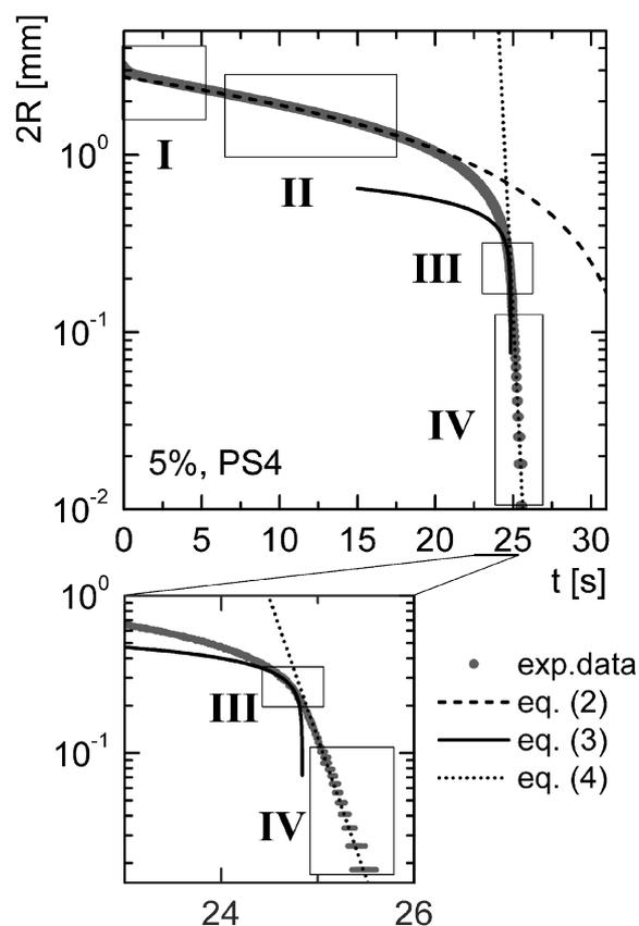
**Fig. 2.** Evolution of the mid filament diameter  $2R$  as function of time  $t$  for a 5 wt% solution of polystyrene PS4 ( $M_w = 3.84 \cdot 10^6 \text{ g/mol}$ ) in diethylphthalate.
