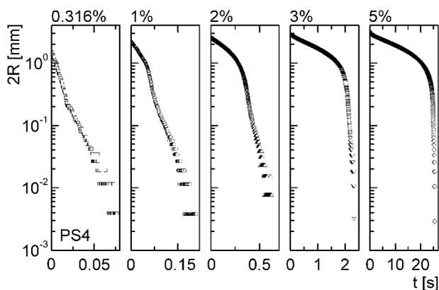
**Fig. 1.** Evolution of the mid filament diameter  $2R$  as function of time  $t$  for solutions of polystyrene PS4 ( $M_w = 3.84 \cdot 10^6 \text{ g/mol}$ ) in diethylphthalate at five different concentrations.
