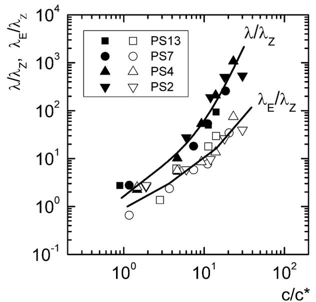
**Fig. 8.** Comparison of the terminal relaxation time  $\lambda$  from oscillatory shear experiments with the extensional relaxation time  $\lambda_E$  experiments (both normalized with the Zimm relaxation time  $\lambda_Z$ ).
