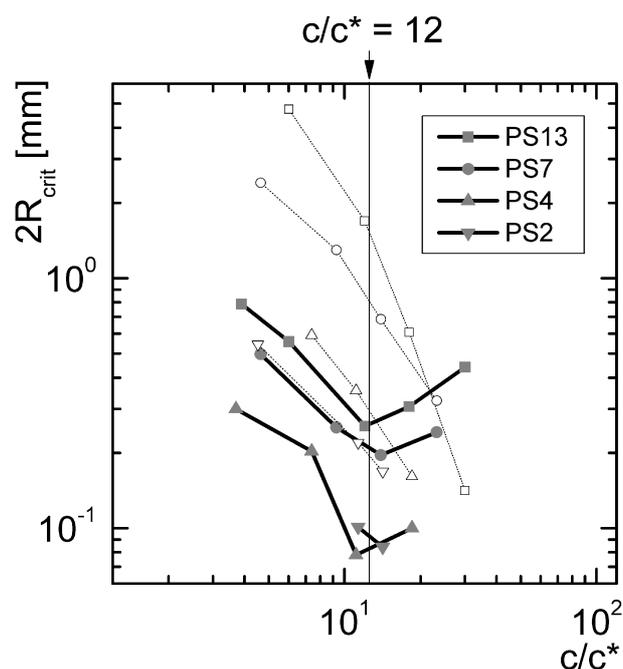
Fig. 5. Critical diameter  $2R_{crit}$  (at which a transition from the visco-capillary to the elastocapillary balance is observed) as a function of the overlap parameter  $c/c^*$  for the different polystyrene in DEP solutions (closed symbols are experimental values, open symbols from eq. (10)).
