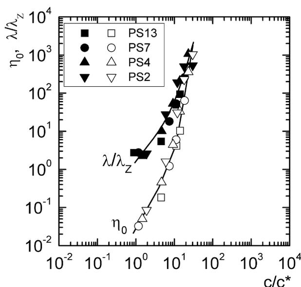
**Fig. 7.** Zero-shear viscosity  $\eta_0$  (open symbols), and terminal relaxation time  $\lambda$  from oscillatory shear experiments (normalized with the Zimm relaxation time  $\lambda_z$ ) (closed symbols), as a function of the overlap parameter  $c/c^*$  for the different polystyrene in DEP solutions.
