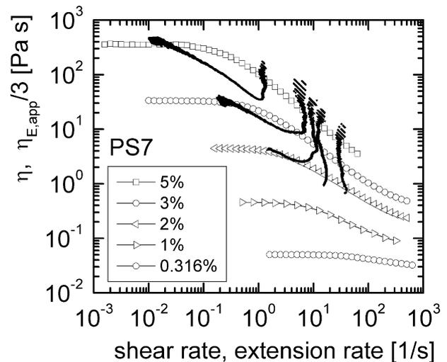
**Fig. 9.** Comparison of the steady shear viscosity  $\eta$  as a function of the shear rate  $\dot{\gamma}$  (open symbols), with the transient, apparent extensional viscosity  $\eta_{E,app}$  as a function of the extension rate  $\dot{\epsilon}$  (small filled symbols) for solutions of polystyrene PS7 ( $M_w = 7.11 \cdot 10^6$  g/mol) in diethylphthalate at five different concentrations.
