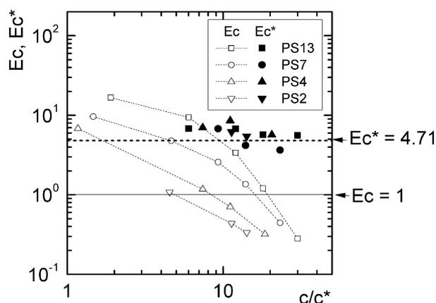
**Fig. 6.** Elastocapillary number  $Ec$  of eq. (7) (open symbols), and local elastocapillary number  $Ec^*$  from eq. (8) (filled symbols) as a function of the overlap parameter  $c/c^*$  for the different polystyrene in DEP solutions.
