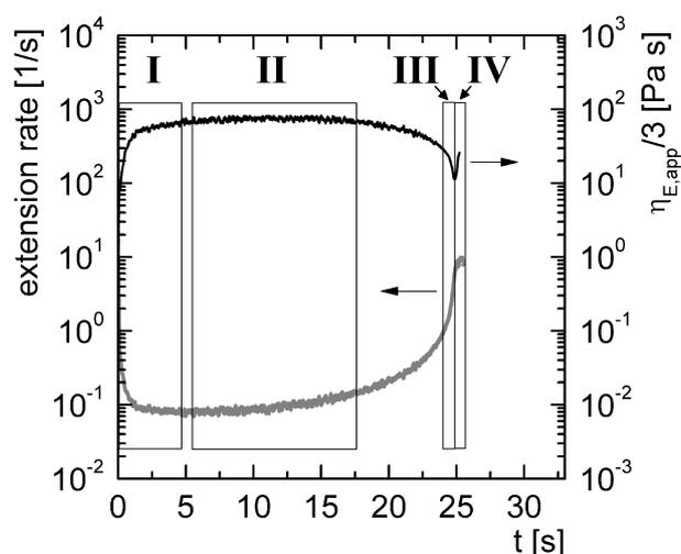
**Fig. 3.** Extension rate  $\dot{\epsilon}$  and apparent extensional viscosity  $\eta_{E,app}$  evolution in a capillary breakup experiment for a solution of polystyrene PS4 ( $M_w = 3.84 \cdot 10^6$  g/mol) in diethylphthalate, determined from the thinning data of Fig. 2 via eq. (5) and (6).
